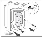
**5.** Open the porthole and remove the polystyrene block fitted on the door seal.
